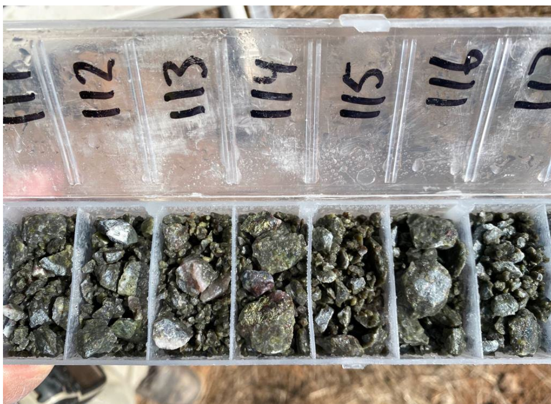
Figure 4: Veined-hosted sulphide mineralisation; sphalerite (brown-purple), galena (silver grey) and chalcopyrite (golden yellow) in RC hole BM001 from 111-117m
